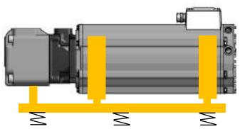
GVM motors have been designed for an horizontal mounting (see §4.2). Considering the above schematics, GVM motors have to be supported on their rear side. For alternative mounting positions, please contact Parker.
