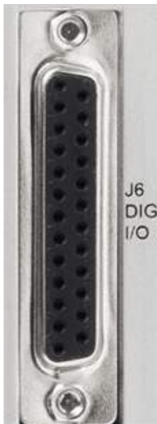
Figure 4-11. J6 - Digital I/O Connector
