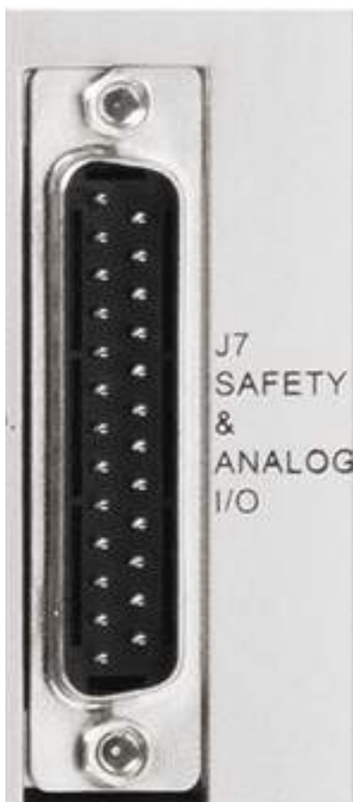
Figure 4-17. J7 - Analog & Safety I/O Output Connector
