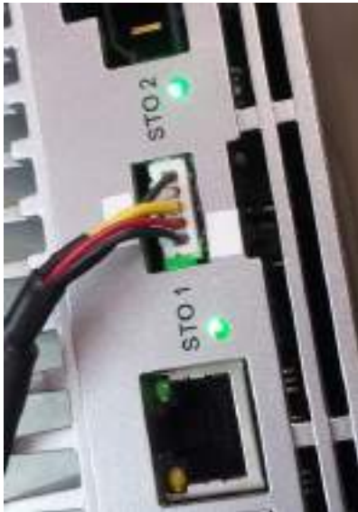
Figure 8: STO J2 Connector and its LEDs
