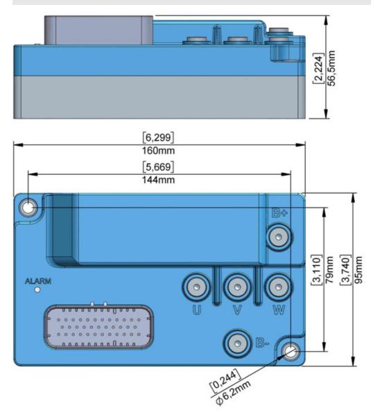
Fix the controller with all the screws on a metal surface (aluminum if possible) to reduce the heat and so for longer working time.
