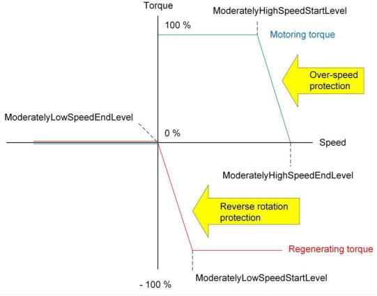
Figure 30 Motor current limitation due to motor speed (no torques at reverse speed)
