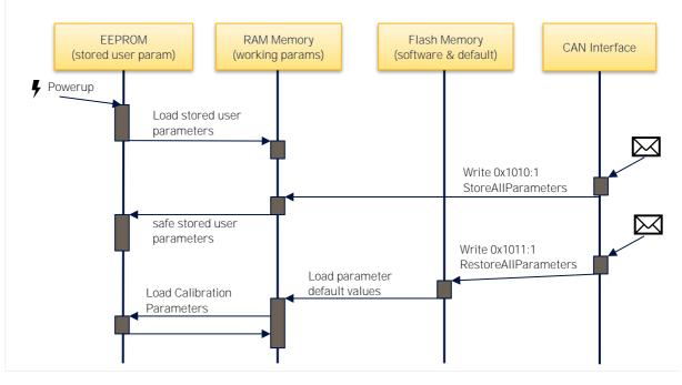
Figure 2 Parameter Access and Flow
