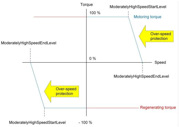
Figure 29 Motor current limitation due to motor speed (full torques at reverse speed)
