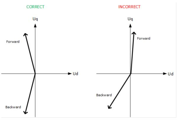
Figure 35 Examples of correct and incorrect alignment
