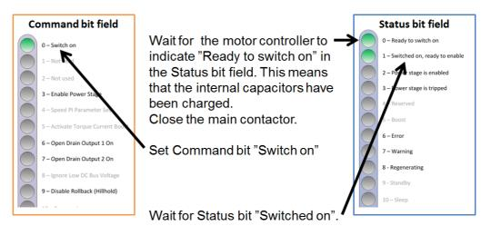
Figure 38 Switch on procedure
