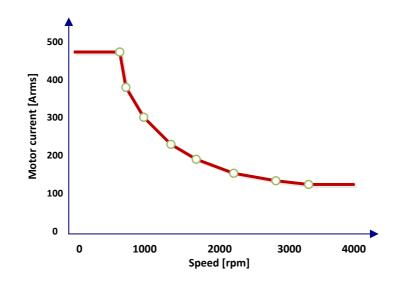
Figure 25 Example of Best Performance Curve (BPC).Speed and Motor Current points are set in 0x2140:1-8 and 0x2141:1-8
