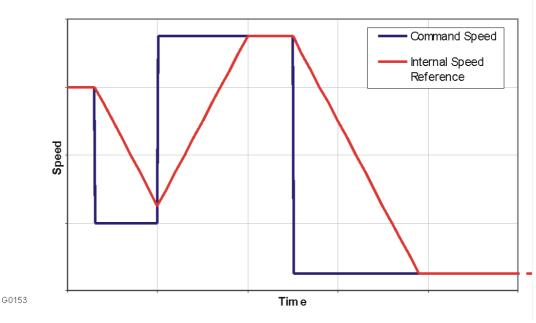
Figure 20 The basic speed ramp
