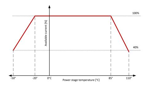
Figure 26 Graphical view of how power stage temperature limits the available motor current
