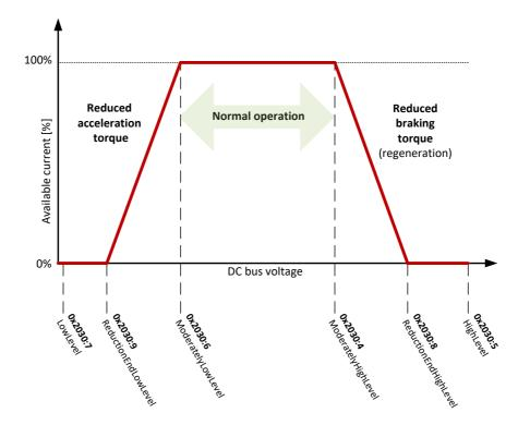
Figure 27 Graphical view of how DC bus voltage level could affect the available motor current
