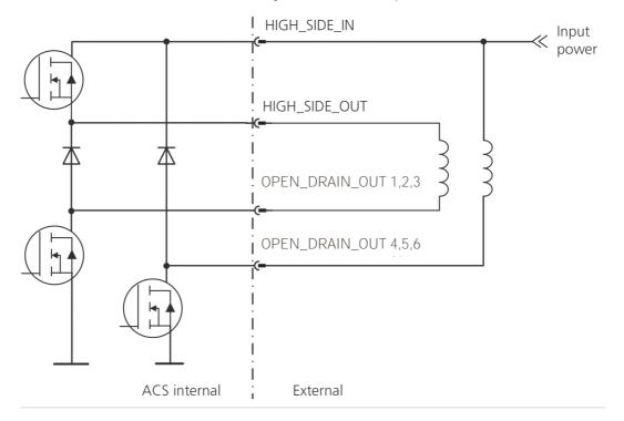
On PDO error OPEN\_DRAIN 1, 3 and 5 are switched off, the others are not affected by PDO errors.
