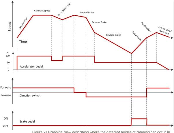
Figure 21 Graphical view describing where the different modes of ramping can occur in a Parameter Controlled Ramp setup. The accelerator pedal input can also be seen as the commanded speed value from a PDO
