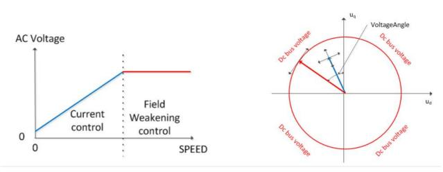
Figure 11 Field weakening control mode
