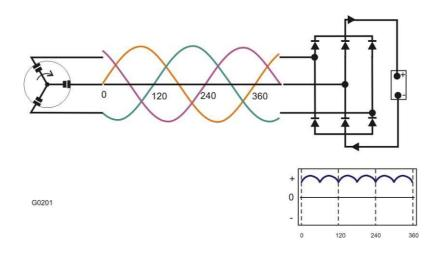
Figure 34 Current Flow during Regeneration
