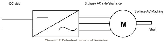
Figure 15. Principal layout of inverter.
