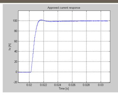
Figure 7 Current step response that is approved. The rise time is adequate and the overshoot is only a few percent.
