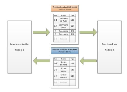
Figure 37 PDO communication between Master (Node 1) and (Traction Node 3) has started. Node 3 is used as an example.
