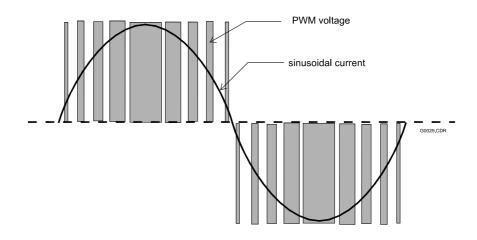
Figure 33 Pulse Width Modulation
