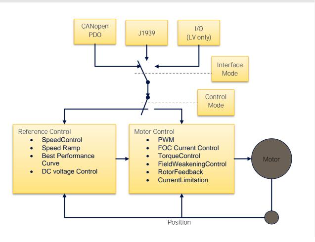
Figure 3 Overview of the motor controller control structure
