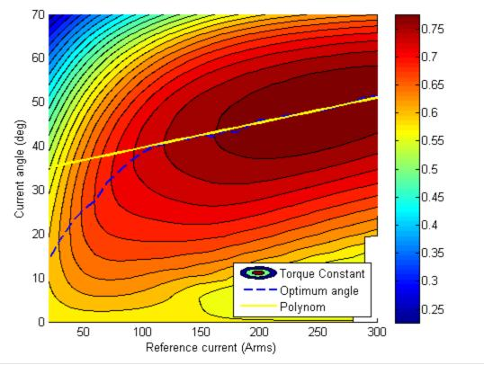
Figure 12 Optimum current angle as function of total current for a PMAC motor
