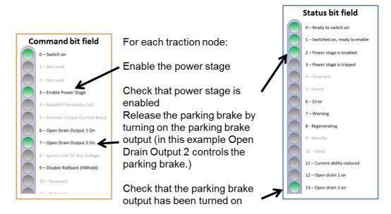
Figure 39 Enabling of power stage and (if used) releasing the parking brake
