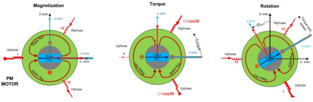
Figure 5 Field Oriented Control for PMAC motors
