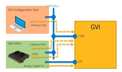
Figure 1 GVI Communication Interface for configuration and operation
