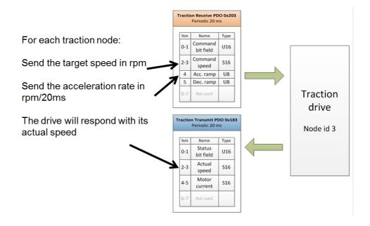
Figure 40 Speed reference command, accelerating
