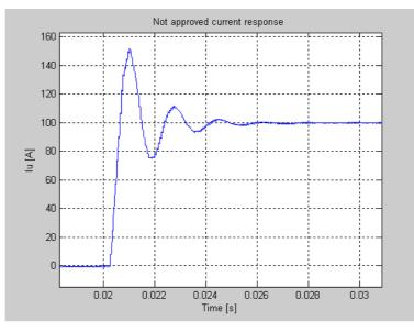
Figure 8 Current step response that is not approved. The rise time is too low, the overshoot is around 50% and is also followed by a significant undershoot.
