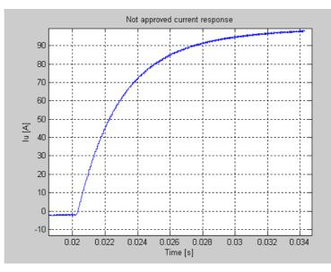
Figure 9 Current step response that is not approved. The rise time is too long.
